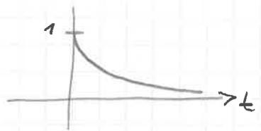
$$F(\omega) = \int_{-\infty}^{\infty} f(t) e^{-i\omega t} dt = \int_0^{\infty} e^{-\alpha t} e^{-i\omega t} dt = \int_0^{\infty} e^{-(\alpha + i\omega)t} dt =$$
